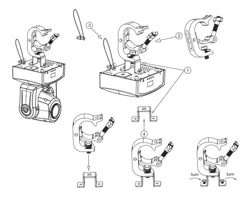
Screw one clamp via a M12 screw and nut to the included bracket. Attach the bracket using the included screws to the bottom of the Stinger Spot. Attach the eyehole screw to the bottom of the base and pull the safety-cable through the screw and over the trussing system or a safe fixation spot. Insert the end in the carabine and tighten the safety screw.
