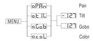
To enter the home position adjustment menu, press the ENTER button for at least 5 seconds. In this submenu you are able to adjust the original position of the pan position, tilt position, color wheel position, and gobo wheel position.
